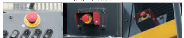
Emergency engine stop switch
