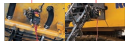
Emergency engine stop switch
