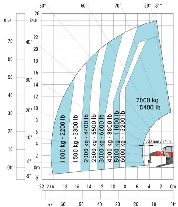
Machine on lowered stabilisers with winch 6000 kg (Metric) Machine on lowered stabilisers with winch 7200 kg (metric)
